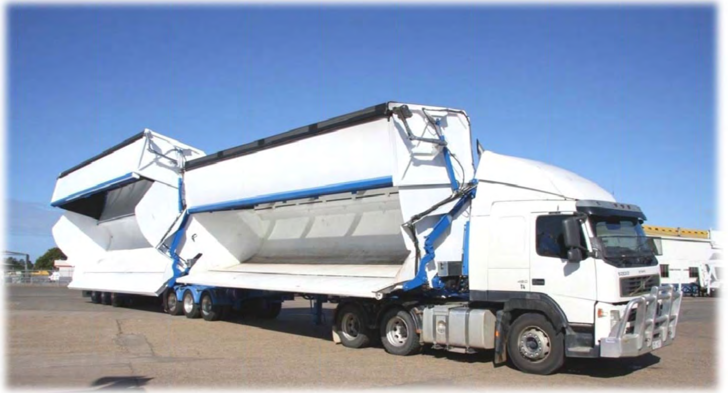
HIGH VOLUME SIDE TIPPER IN B-DOUBLE CONFIGURATION.
