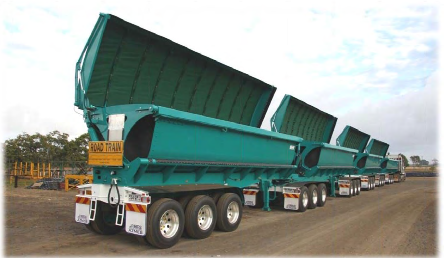
QUAD ROAD TRAIN CONFIGURATION ON TRI AXLE TRAILERS & TRI AXLE DOLLIES.
