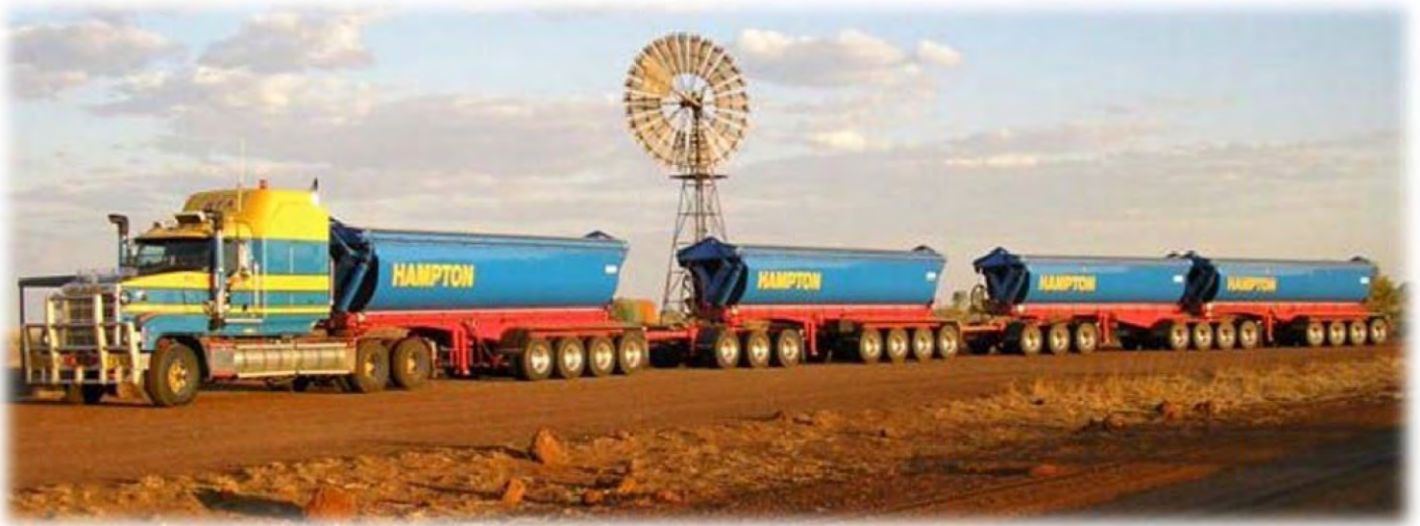
QUAD ROAD TRAIN CONFIGURATION ON QUAD AXLE TRAILERS & TRI AXLE DOLLIES.
